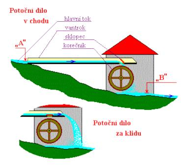
This work has been used in the past only for the sub-offices (local mills, churns, and the output washboards), which used a local creek flowing from the side. Water flows continuously, without the possibility of accumulation.
