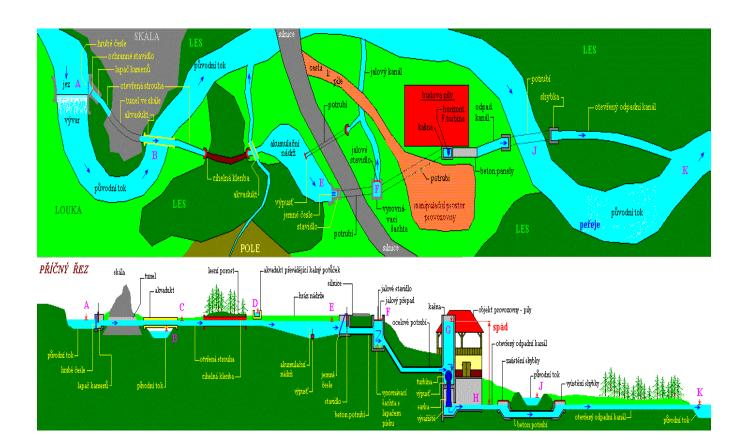
This work was established in the 18th century as a saw mill. The drive was water wheel, the working machine was a saw mill machine. Water was collected at the weir at the point "B". Drive skirted the forest along the river; the accumulation tanks were not needed. There was a **wooden vantrok** on the poles from the road to the saw. Water was returned in the point" J ".
