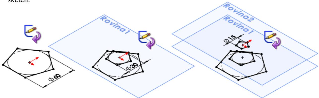
2. Construct parallel helping **Plane 1** to **Upper** plane in distance of 12 mm. Validate the plane. Draw the sketch of pentagon profile in the plane with the size of inscribed circle 30 mm. Close the sketch.
