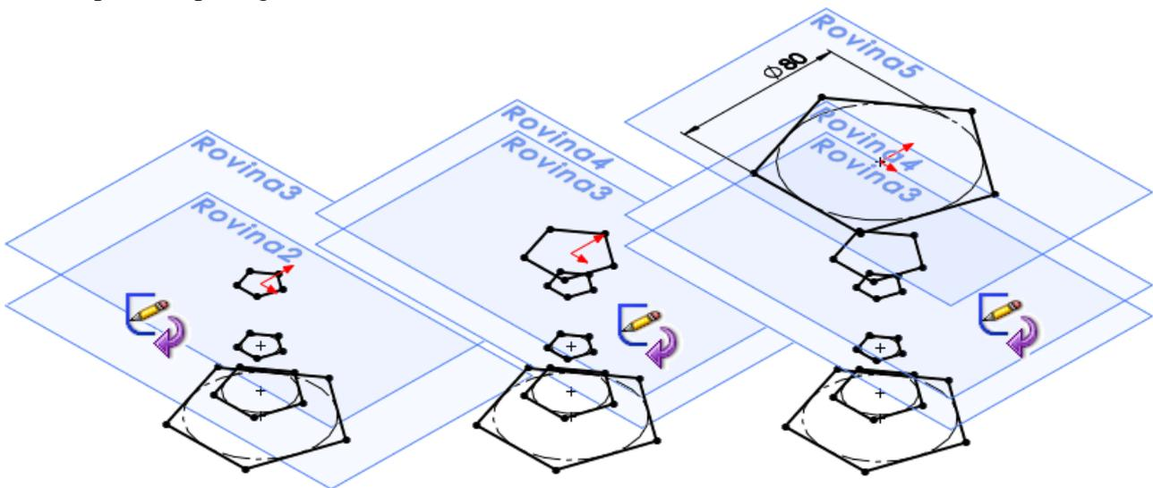
4. Construct parallel helping **Plane 3** to **Plane 2** in distance of 30 mm . Validate the plane. Copy Sketch 3 onto Plane 3. Close the sketch.
