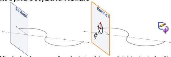
4. Choose **Adding by drawing on curve from** the choice of elements. Label the sketch of profile (usually it is written in Property Manager automatically). Label the sketch of curve as line. If the line is drawn correctly (every curves are tangential) and profile has correct size, preview is displayed and check it.
