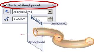
Lines are often made by curves (spiral, helix) – in the choice of Elements. The base of these curves is the sketch of circle.
