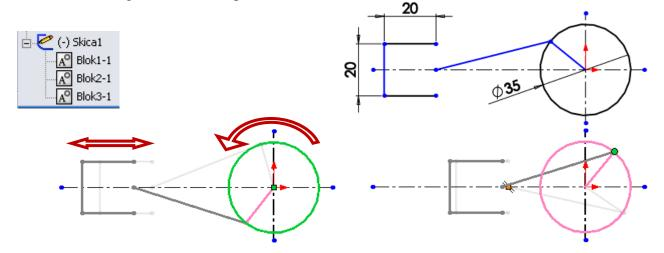
3. Independently create and animate moving of star- shaped engine with three rollers
