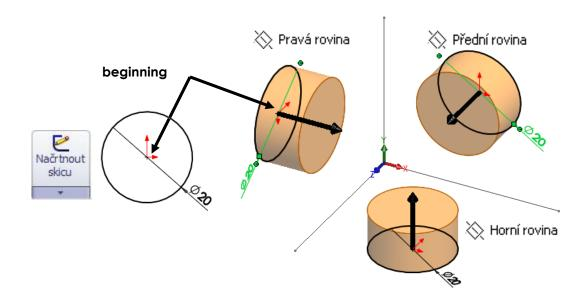
Drawing of entities is possible only in active plane. This sketch active plane you can recognize according to beginning red arrows. After opening of active sketch in required plane choose entities commands from menu for drawing (left mouse button - LMB).
