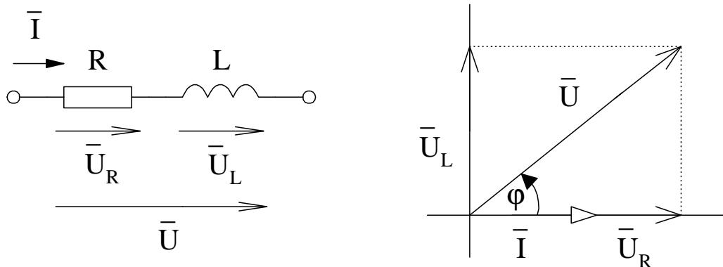
$$\bar{U} = \bar{U}_R + \bar{U}_L \quad \bar{U}_R = R\bar{I} \quad \bar{U}_L = j\omega L\bar{I}$$
