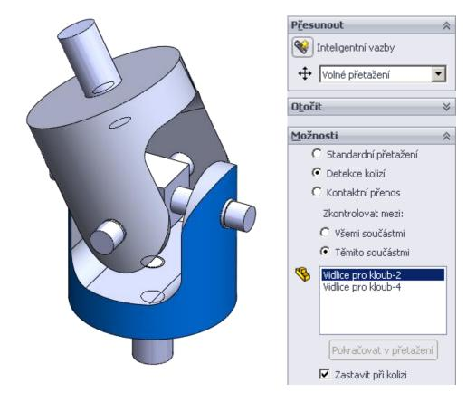
Oscilate fork of the joint in two directions
