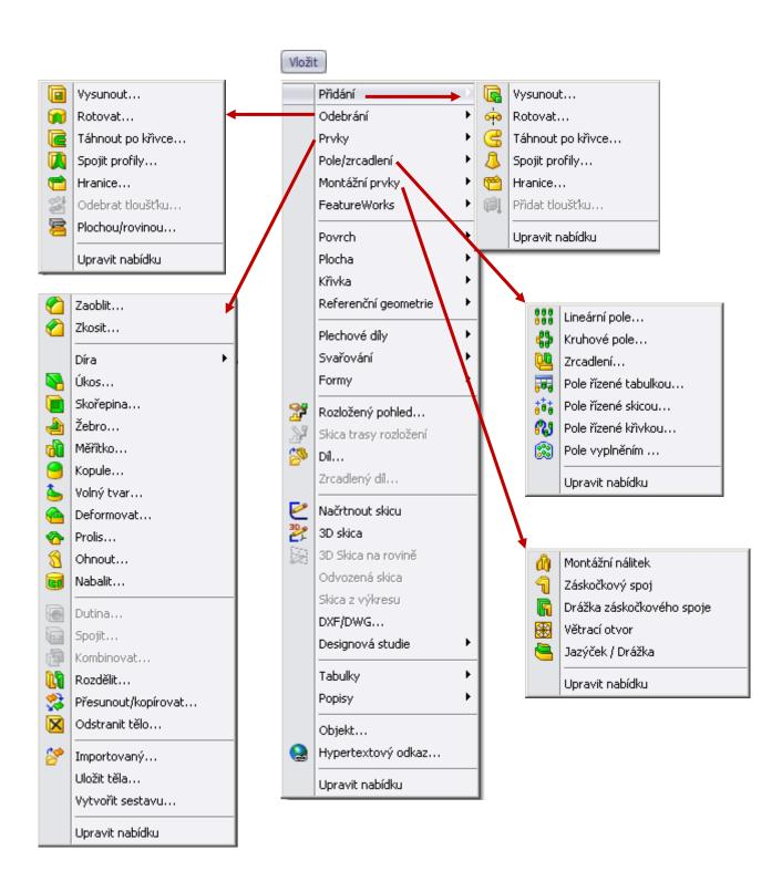
**Elements** are particular geometrical shapes appropriate combination of which can help us making required model - a Part . For some elements the sketch is the base (adding of putting out, taking of putting out ), for other elements capacity solid figure must be prepared. Elements are divided into basic and dependent.
