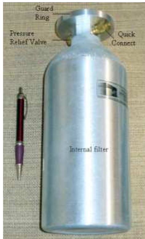
Obr. 8.22 . CL-910 Metal hydride hydrogen storage container
